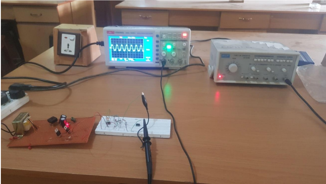
Figure 3: The measurement setup of the Wienbridge oscillator on a breadboard
