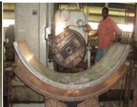
Figure 4: Ball Mill Trunnion Bearing
