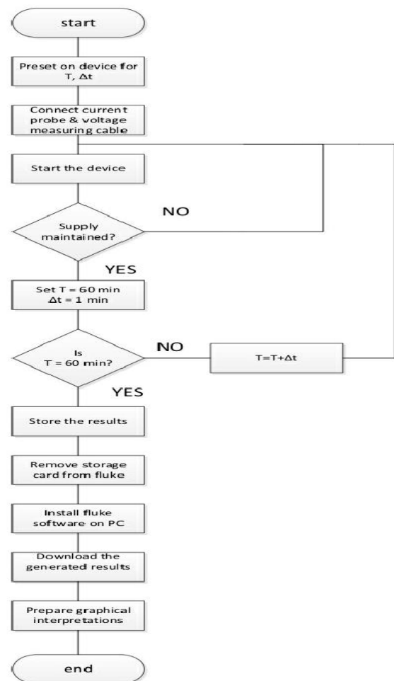
Figure 3: The flow process of DT power analysis using power quality and energy Analyzer
