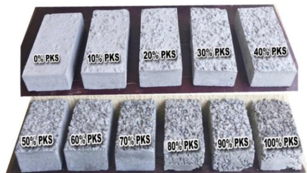
Figure 2: Eleven (11) samples of concrete interlocks with varying percentage ratio of PKS.
