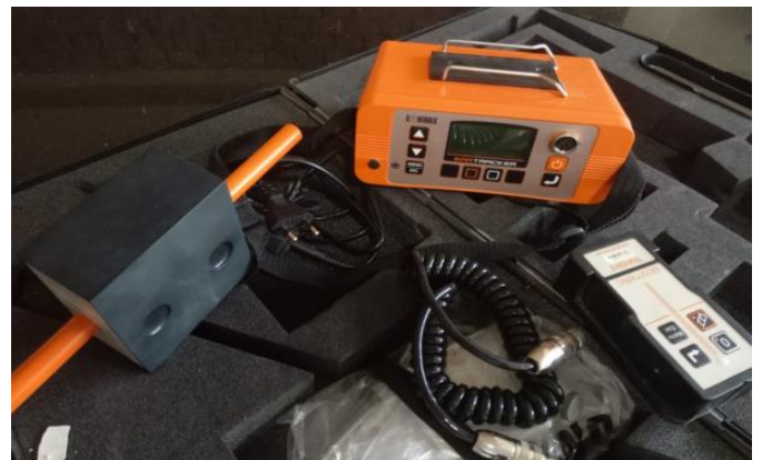
Figure 6: Covermeter device used for the study
