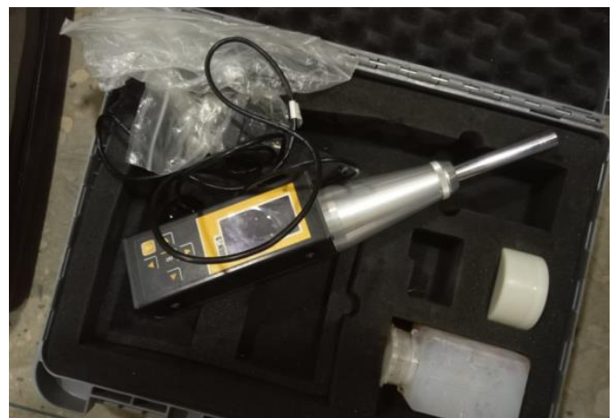
Figure 7: Digital Rebound Hammer test kit used for the study
