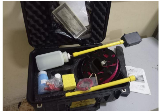
Figure 11: Half- Cell Potential Equipment Kit used for the Study
