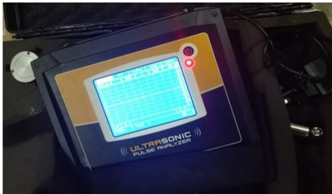
Figure 9: Ultrasonic pulse velocity device used for the study
