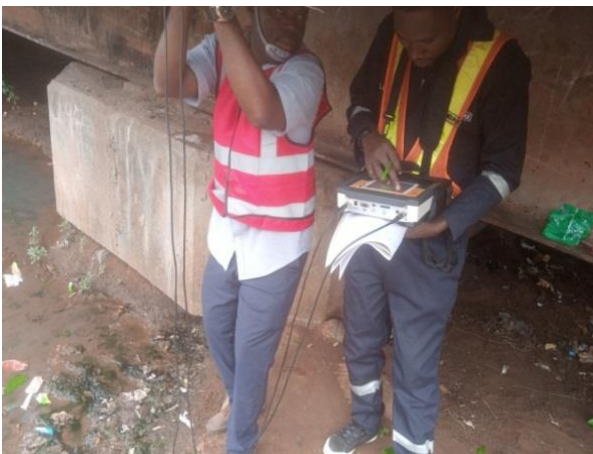
Figure 10: Determination of UPV values of the Orogodo Bridge deck
